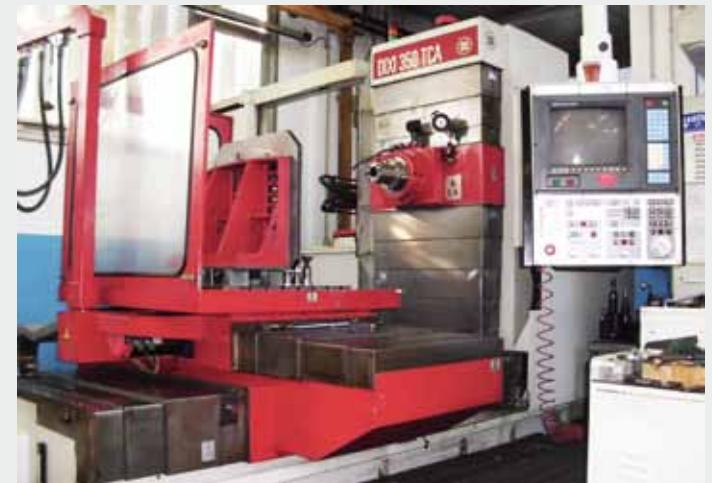
The Boring machine department is made up of traditional (Genevoise) and 4/5 axes CNC (SIP, DIXI) boring machines, with both vertical and horizontal spindle and high structural precision. Highly experienced personnel manage these equipment, specialized in the execution of unique parts or of small series which require special manufacturing accuracy. The department is temperature controlled.
