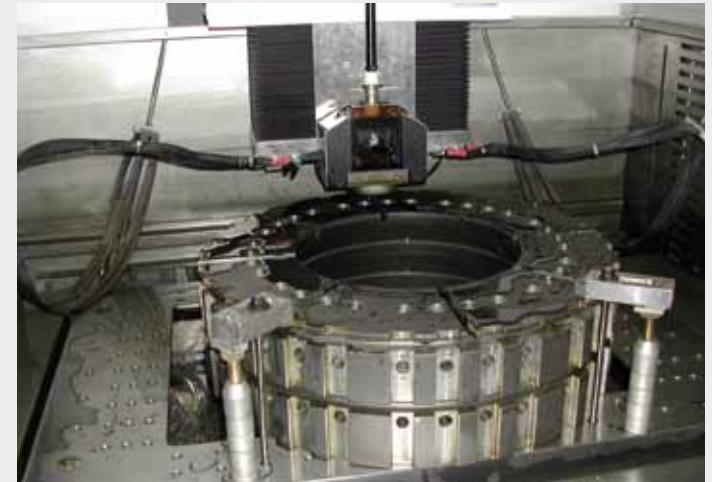
The EDM (Electro Discharge Machining) department provides a modern "AgieCharmilles CUT30P" wire-cut machine which can quickly perform high-precision machining while ensuring an excellent surface finishing. It can work maximum dimensions of 1050x800x350mm and easily implement shapes which would be hardly created by conventional machines.
