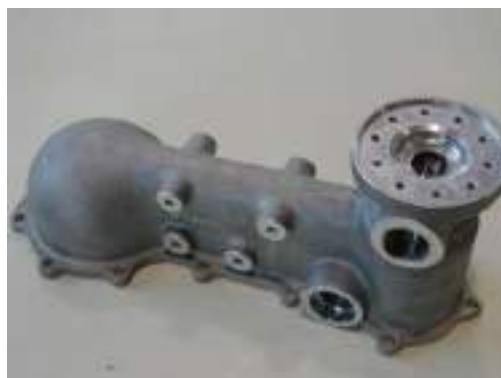
Helicopter support oil level
